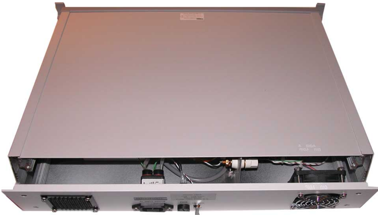
Figure 4.3 Rear panel tilted down
