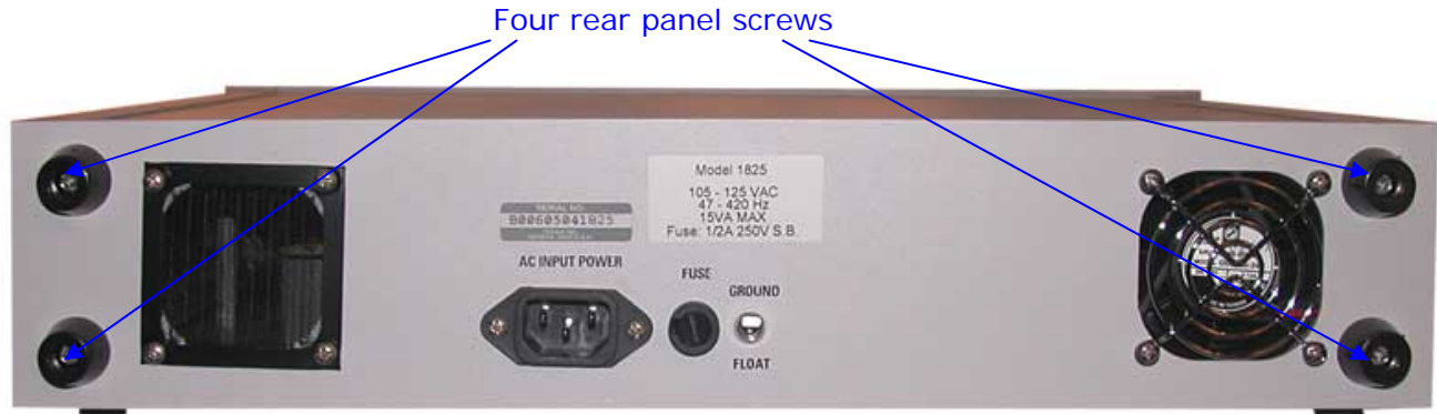
Figure 3.2 Location of four rear panel screws
