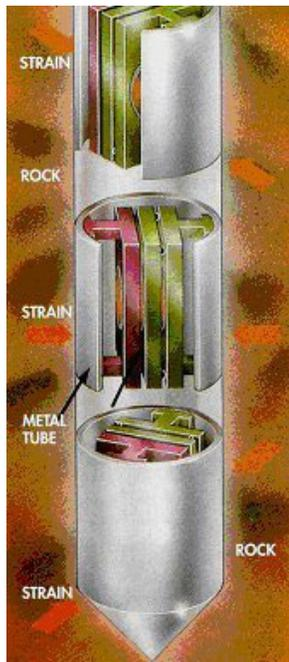
*Figure 5 – The GTSM Tensor Strainmeter as installed in the borehole.*
