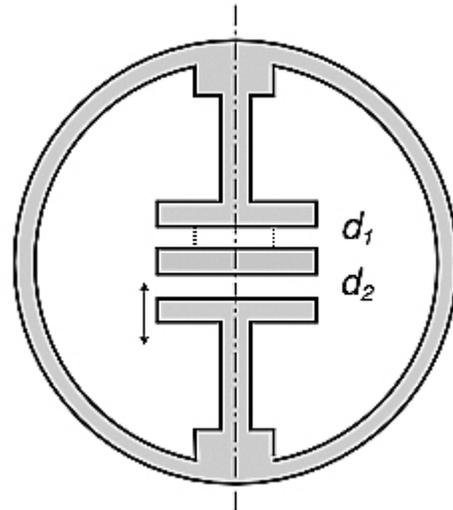
*Figure 3 – Mechanical representation of one axis of the of the strain element. As distances  $d_1$  and  $d_2$  vary with rock deformation, the capacitive output will also vary.*
