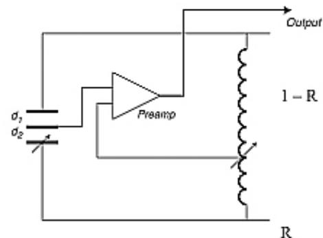
*Figure 4 – Electrical representation of the strainmeter. The TEGAM ratio transformer is shown as “R” in the schematic. The initial output of the device is set at zero.*
