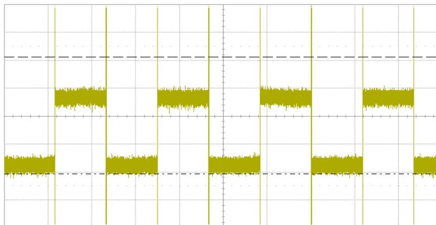
Graph 2 - 1750's test signal in an inductive measurement (5 mV/div)
