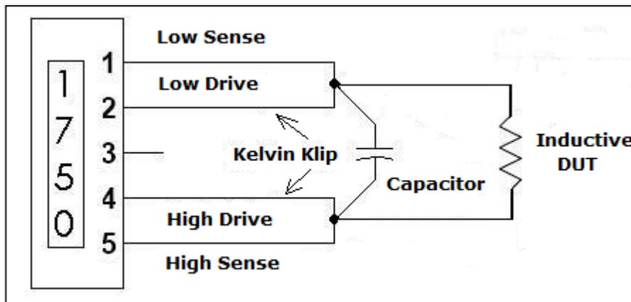
Figure 1 - 1750's setup for an inductive DUT.
