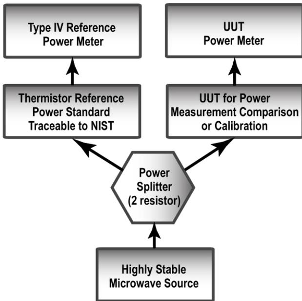
Figure 1 – Block diagram of a Direct Comparison System.
