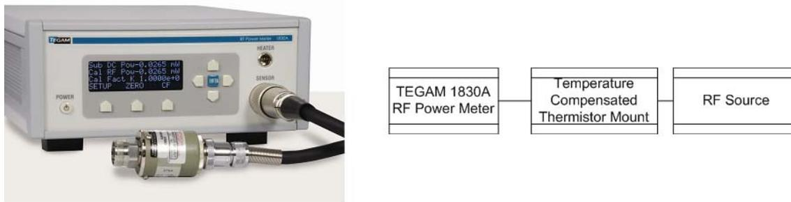
Figure 3 - TEGAM 1830A Method for Measuring Thermistor Mounts
