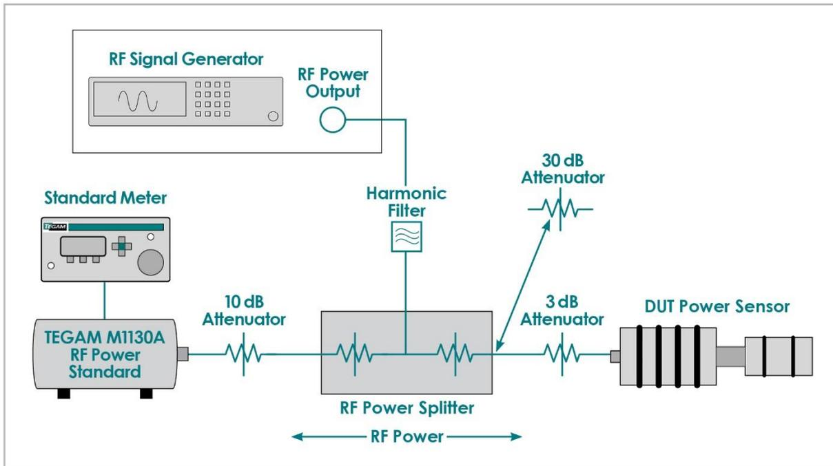
**Figure 2** Complete Linearity Verification Configuration
