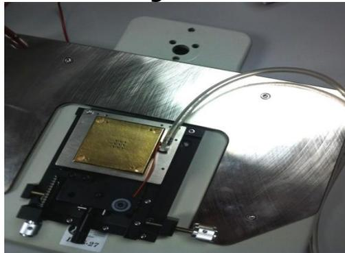
*Figure 2 - LMS-2709 Vacuum Clamping Stage with ferromagnetic plate.*
