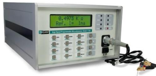
*Figure 1 – The TEGAM Model 1740 Microohmmeter employs a four-wire Kelvin lead configuration to achieve a basic accuracy of 0.02% with 1  $\mu\Omega$  resolution. The TEGAM 1740 is fully programmable via its RS-232 and GPIB interfaces (model 1740/GPIB) and is PLC compatible.*
