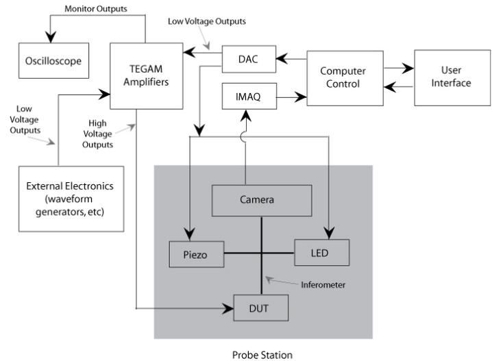
Figure 4 – Professor Ashurst, Auburn University, uses a desktop computer containing a National Instruments DAC card to feed signals to the TEGAM amplifier and the OPTOPro controls. The profiler's flexibility lets researchers use different external generators, monitors, and data acquisition systems as needed for their unique studies.
