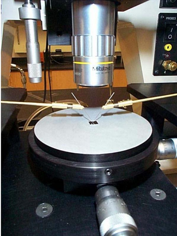
Figure 3 – One major improvement that makes the OPTOPro ideal for MEMS development and characterization is its longer working distance, which allows researchers to more easily attach a variety of different probes. Another is the new TEGAM amplifier that delivers up to 200 V, the highest voltage currently available for MEMS research, to actuate the electrostatic features of the MEMS devices.
