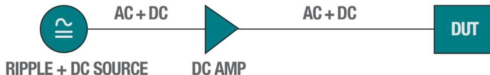
*Figure 4 - Using the TEGAM 2348 Power Amplifier with an arbitrary waveform generator can greatly simplify the test setup for PSRR measurements.*
