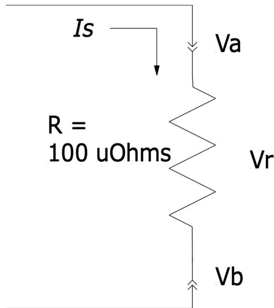
*Figure 2: Thermal contact potentials can totally throw off a low-resistance measurement.*
