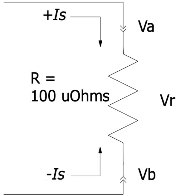
*Figure 3: Making two measurements and averaging the results completely eliminates the effects of thermal contact voltage on low-resistance measurements.*
