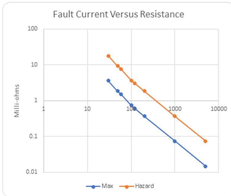
Figure 1: Use this chart to determine the maximum bond resistance for an estimated fault current.
